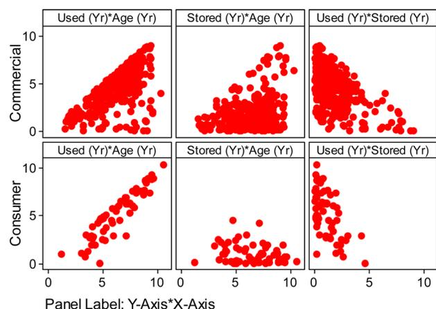
**Fig. 6 Scatter plot of hard drive life characteristics**
