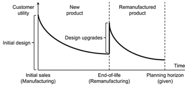
Figure 1. Two components of optimal product design for life-cycle profit: initial product design and design upgrade at the end-of-life stage.
