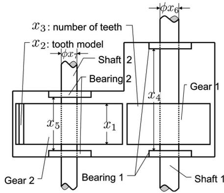
Fig. 7 A schematic of the Golinski's speed reducer
