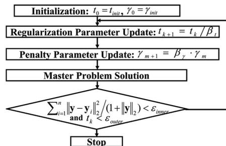
**Fig. 4** The single loop framework of the regularized IPD algorithm
