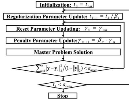
**Fig. 3** The nested loop framework of the regularized IPD algorithm
