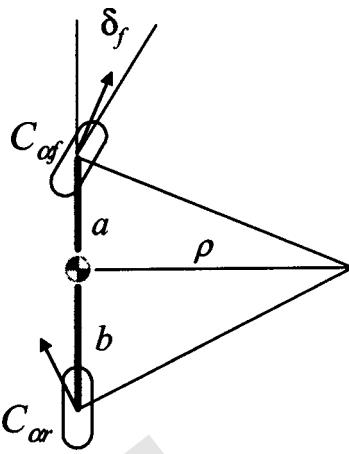
Fig. 5 Cornering of a bicycle model
