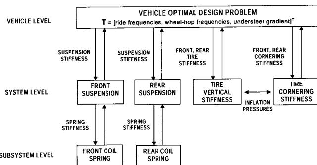
**Fig. 3 SUV chassis design problem structure**
