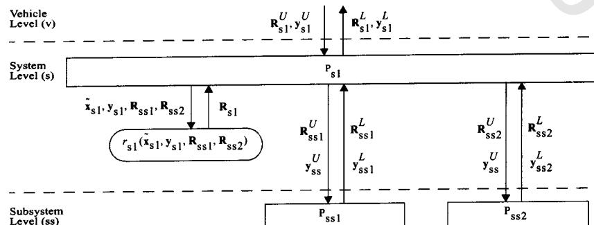
**Fig. 2 Flows from/into the system-level design problem**
