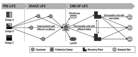
Fig. 1 General recovery structure [1,7]
