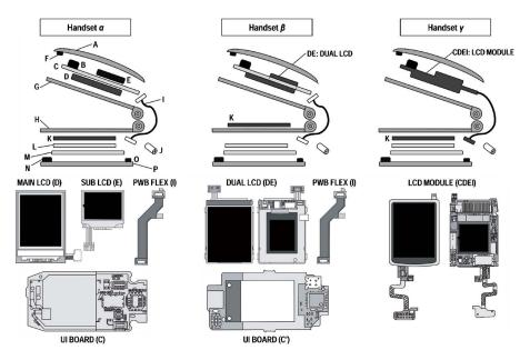
Fig. 4 Three design variants for a clamshell-type handset
