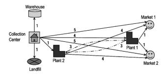
Fig. 5 Logistics network assumption for handset recovery (numbers represent the distance between two facilities; 1 represents a unit distance)
